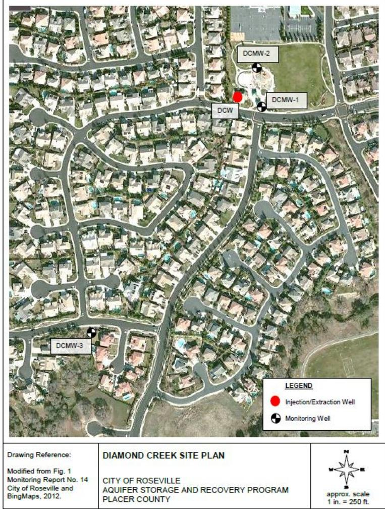
Figure 5: Position of monitoring wells around the Diamond Creek ASR well. (Source: [2])
