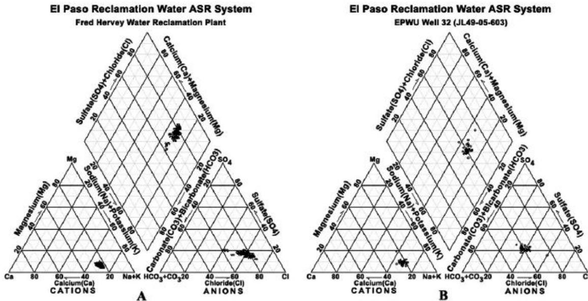
Figure 2: Ionic makeups of the source water (A) and the groundwater near the injection site (B) [1].
