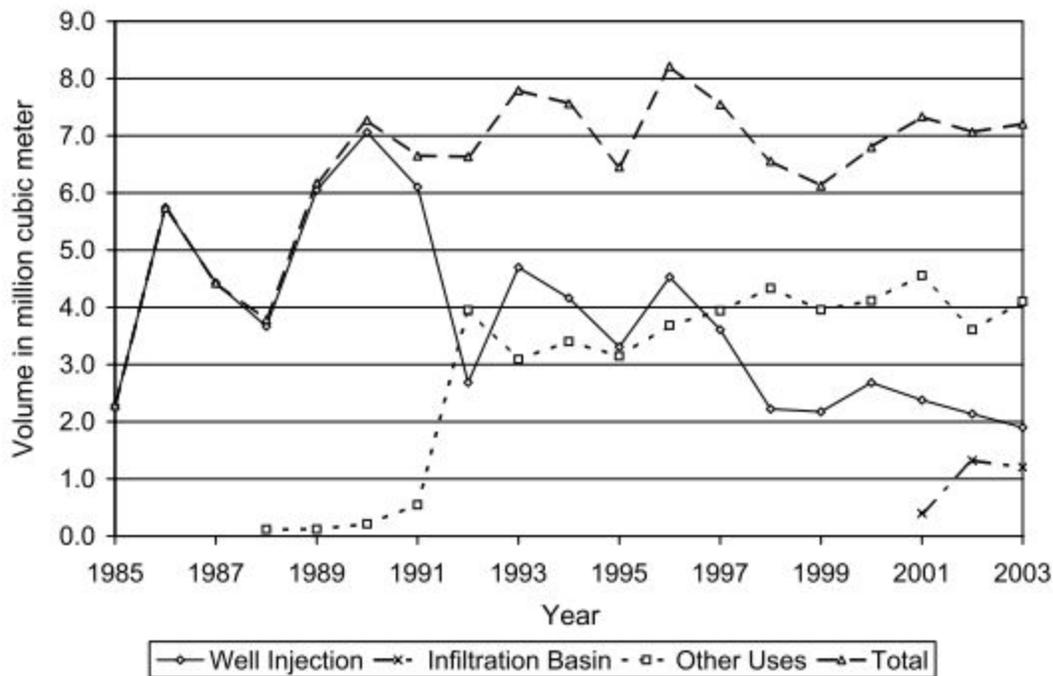
Figure 1: Total reclaimed water production by the Fred Hervey Water Reclamation Plant, and end uses [1].
