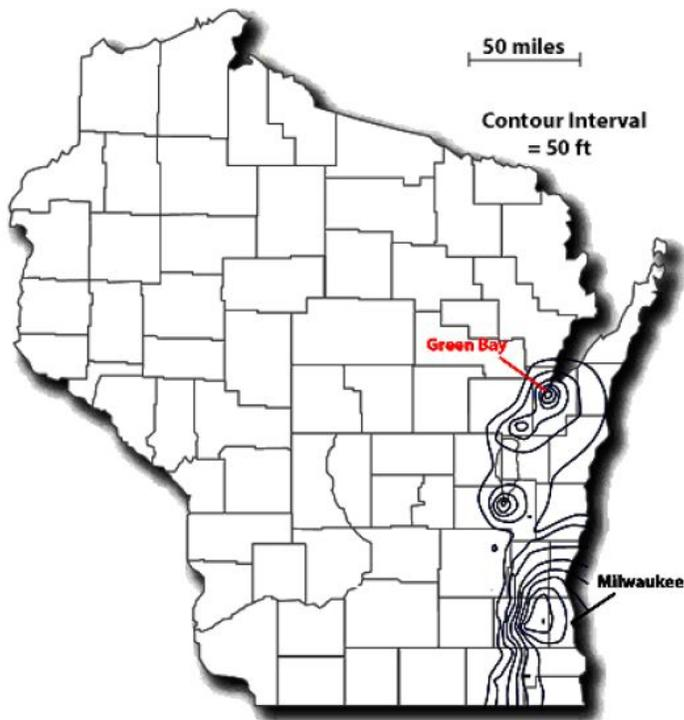
Figure 2: Regional cone of depression network in eastern Wisconsin as of 2000 due to groundwater pumping in the 20<sup>th</sup> century. (Source: [1])
