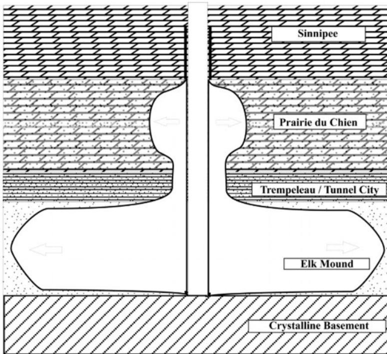
Figure 6: Original conceptual model of the Green Bay ASR flow system. (Source: [1])
