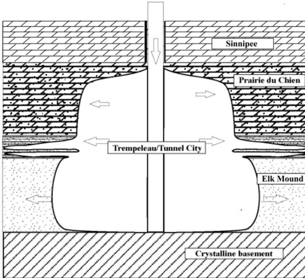
Figure 8: Revised conceptual model of the Green Bay ASR flow system. (Source: [1])
