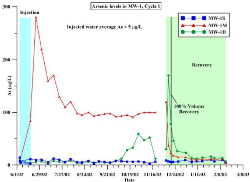
Figure 7: Arsenic levels found during Pilot Cycle 1 in the monitoring well in the Prairie du Chien (MW-1S), Trempeleau-Tunnel City (MW-1M), and Elk Mound (MW-1D) Groups. (Source: [1])
