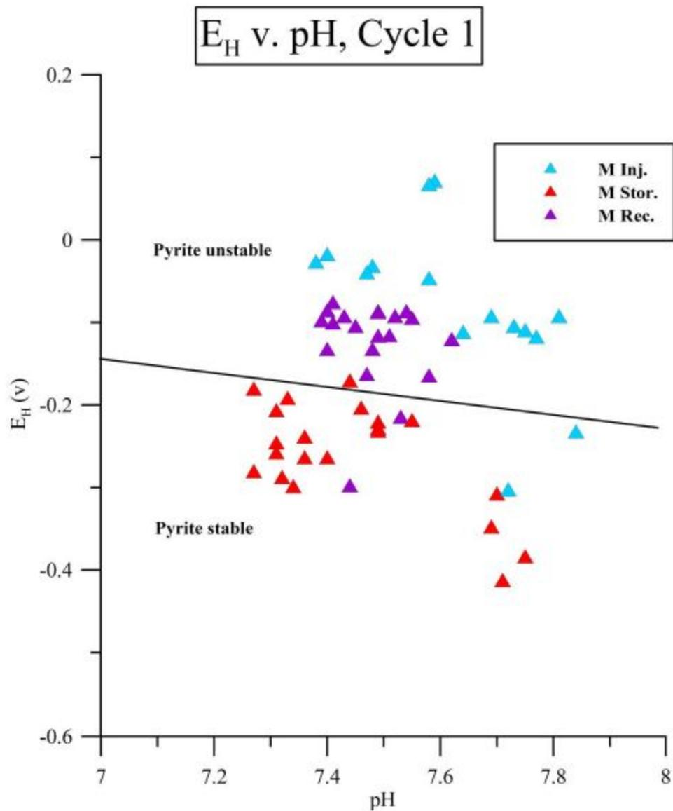
Figure 10:  $E_h$  vs. pH diagram of observations in the Tunnel City Group during injection (M Inj.), storage (M Stor.), and recovery (M Rec.). (Source: [1])
