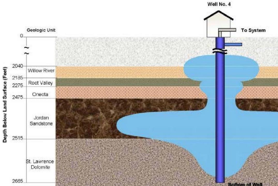
Figure 2: Generalized Stratigraphy for the ASR wells; hypothetical volumes of stored water in the aquifer is represented in light blue (Source: DMWW, 2018).
