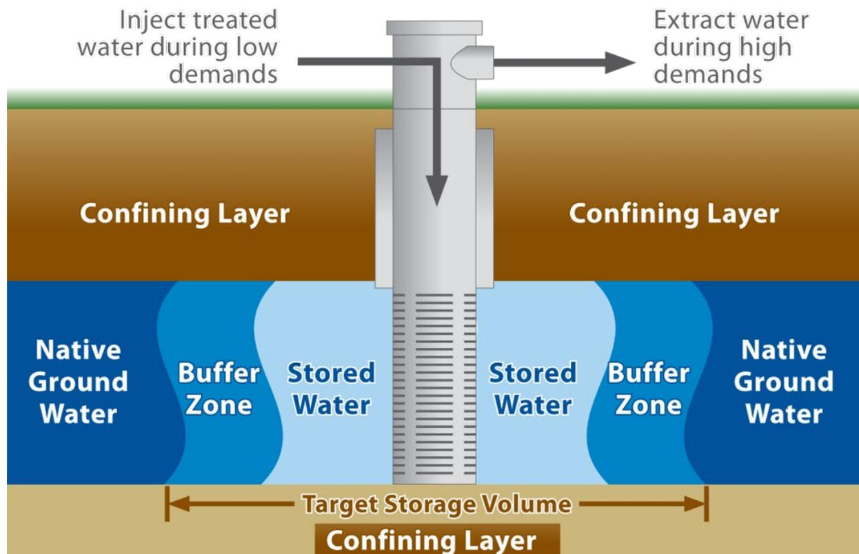
Figure 3. Schematic of injected recharge water, target storage volume (stored water and buffer zone) in confined aquifer, and recovery during high demand periods (Source: TWRD, 2019).
