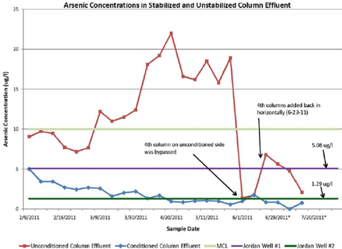
Figure 3: Effects of conditioning pilot plant effluent on arsenic concentrations in column effluent. (Source: [2])
