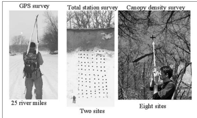
Figure 3. GPS, elevation, and canopy cover characterization of the Blue Earth River Banks. This information was used to interpret and verify the accuracy of the laser data.
