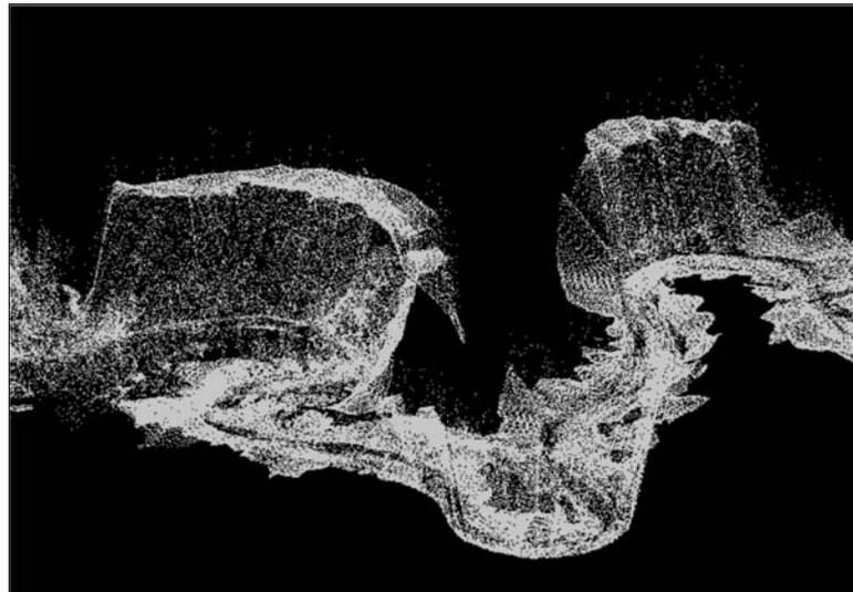
Figure 6. Scanned view of two banks along the Blue Earth River.
