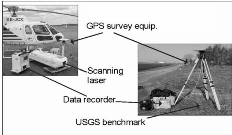
Figure 4. Components of the helicopter based laser system used to scan the Blue Earth River.
